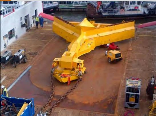
A PLGR can be undertaken by either the cable installation vessel itself, or a suitable third-party vessel such as a tug, small supply vessel, flat back, etc. A typical set of grapnels can be seen in Figure 21, along with a set recovered after it has hooked a wire rope. Normally at least one pass is made along the route of each cable, in which grapnels are hauled in every so often to remove any captured debris.
