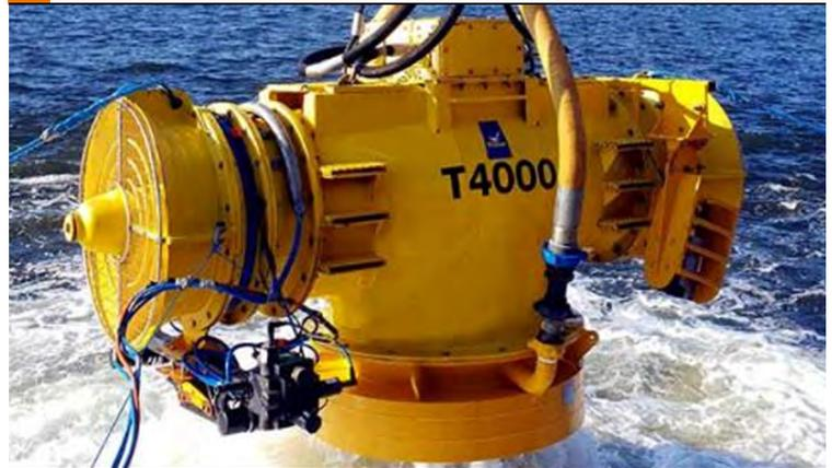
Figure 62. T4000 MFE Fitted with Controllable Positioning System (Courtesy, The Aleron Group).
