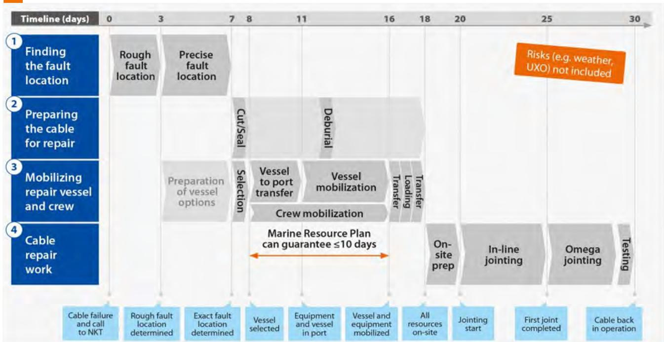
For most cable repairs, two offshore joints must be completed. However, for shore-end replacements, a single joint is normally required and for array cables, the entire cable is usually replaced. A simplified repair sequence is summarized below:
