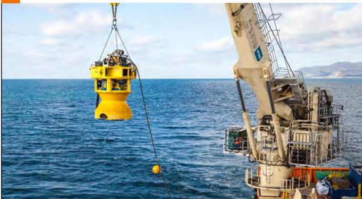
Figure 61. T4000 MFE, Maximum Flow Rate 4,000 L/second and Velocity 10 m/second (Courtesy, James Fisher and Sons).
